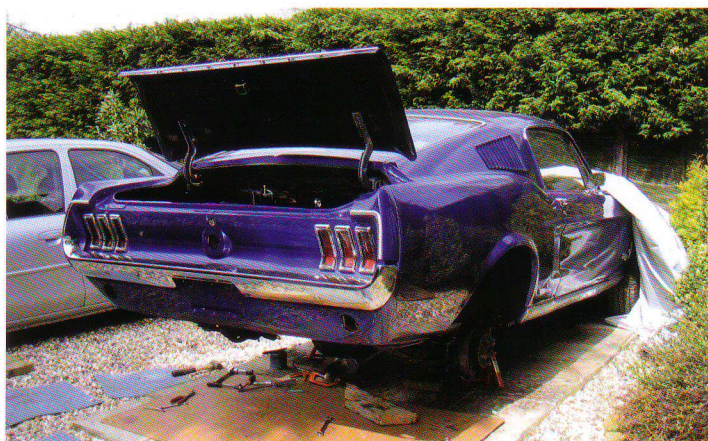
Rebuilt axle and new exhaust being attached - rear drums brakes were renewed
